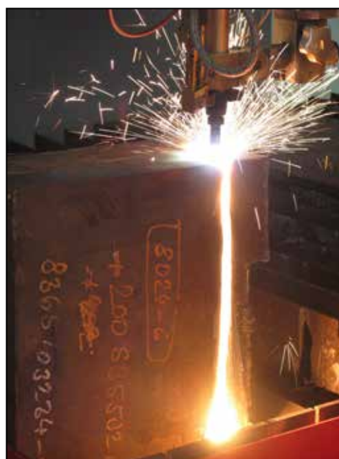
500 mm steel plate cutting
